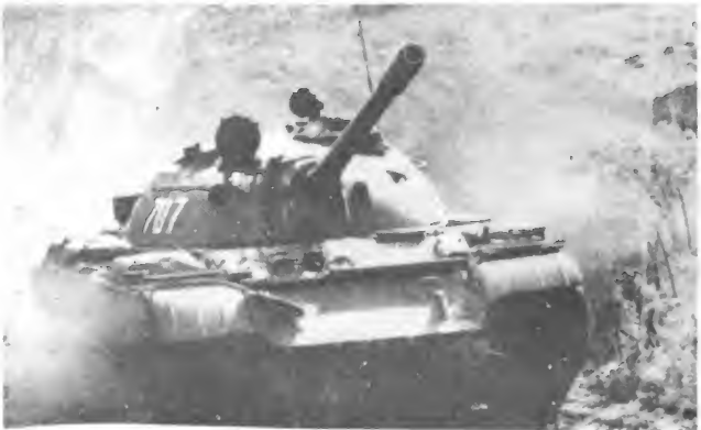
Figure 6-16. T-54/55 medium tanks. T-54 and T-55 tanks exist in numerous variations, all of which mount a 100-mm main gun and can be easily recognized by the large gap between the first and second roadwheels. The T-54A (above) mounts an AA machinegun in addition to coaxial and bow machineguns. The T-55 (below) lacks the AA machinegun.
